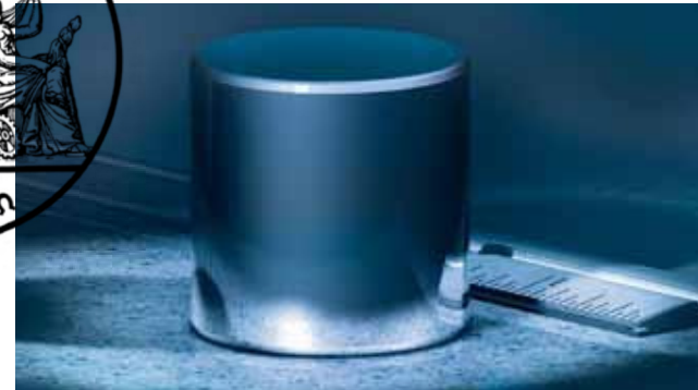
International Prototype Kilogram (IPK) at BIPM, a cylinder made of 90% platinum and 10% iridium.
